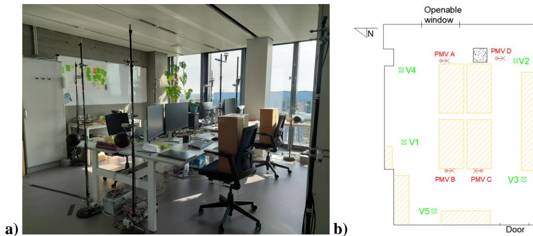
Figure 2: a) The investigated office room with the measurement equipment. b) Location of thermal comfort (PMV, red) and air quality (V, green) poles.
