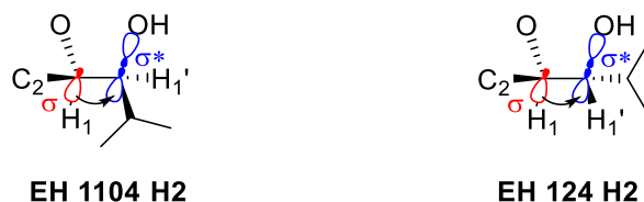
Figure 39: Side view of C1-C1' bond of EH 1104 H2 and EH 124 H2 showing hyperconjugation model for explaining the gauche effect.
