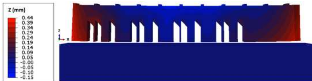
Figure 4.17. FE-predicted component distortion after fully cutting off from the substrate.
