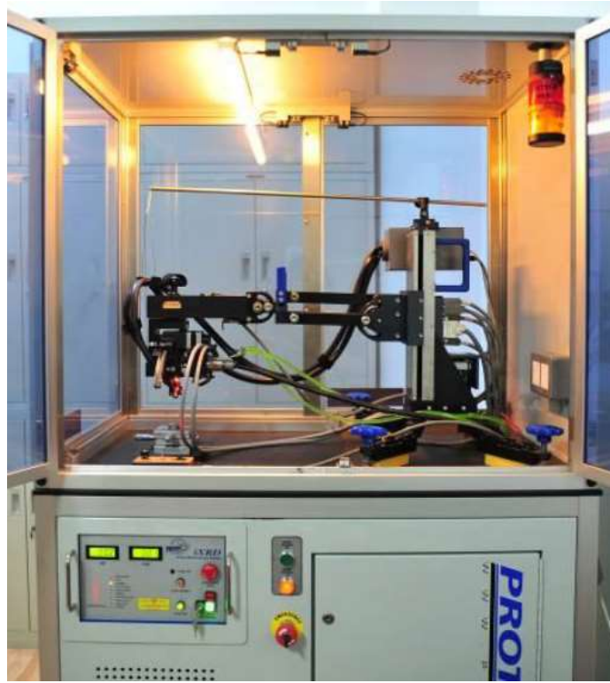
Figure 5.6. Machine used for residual stress measurement.
