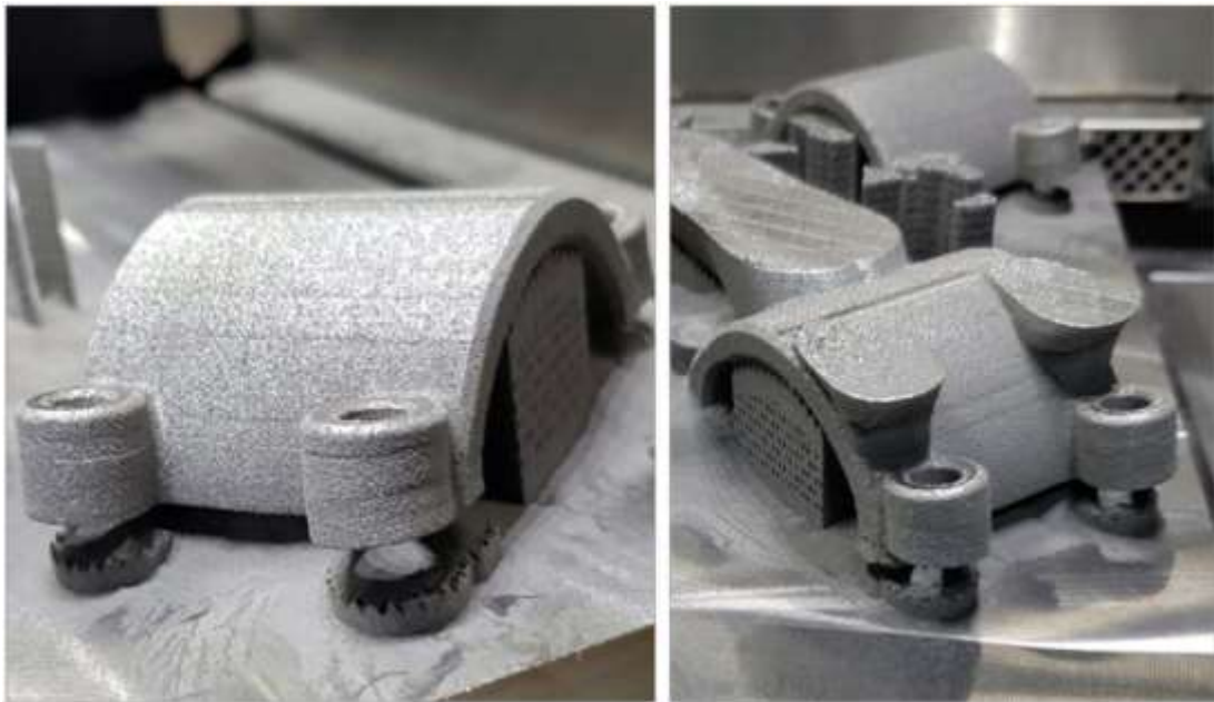
Figure 1.10. Additive manufactured components partly detached from the build due to residual stress (Courtesy of Alexander Liu).
