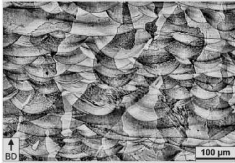
Figure 2.34. Optical micrograph of as-built PBF SS316L [177].
