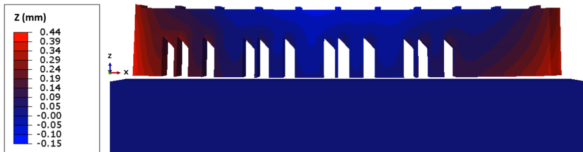
Fig. 17. FE-predicted component distortion after fully cutting off from the substrate.
