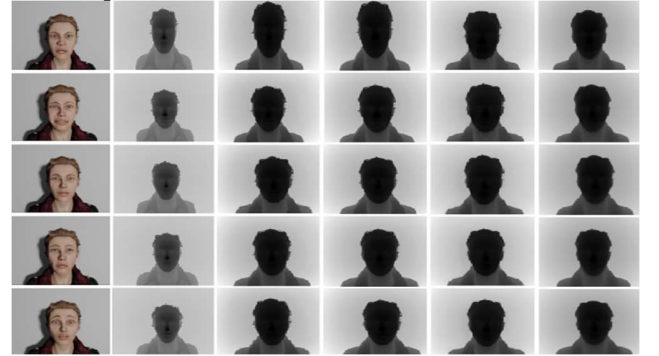
Fig. 14. An example of the qualitative comparison of methods. From left to right: Input, Ground Truth, U-Net, DenseDepth, ResNet and EfficientNet images.
