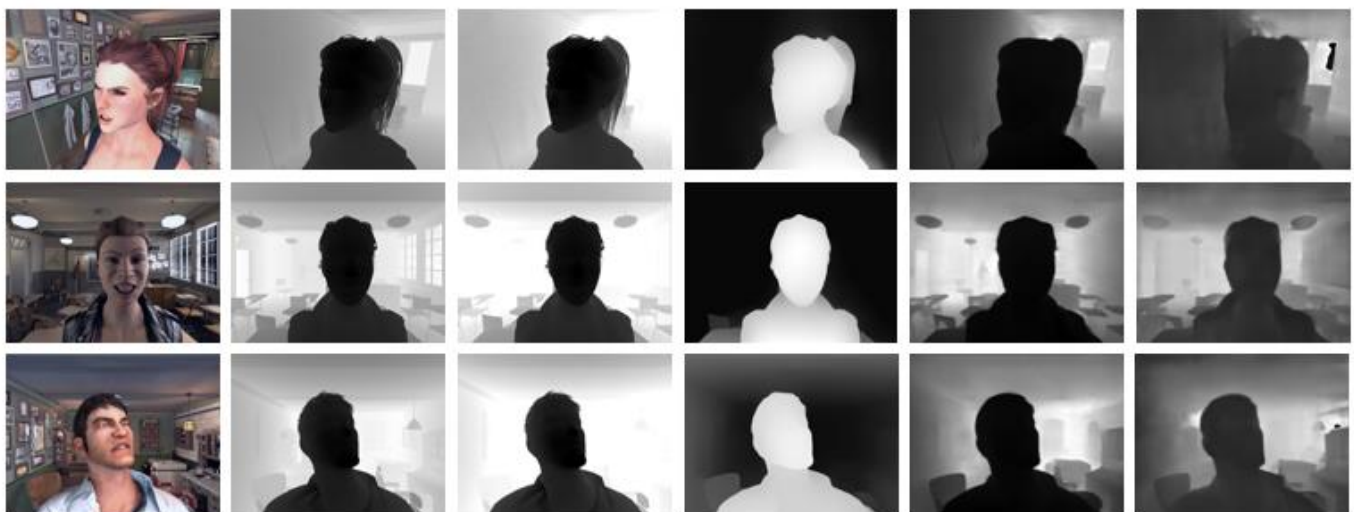
FIGURE 5. From left to right, qualitative results of facial monocular depth estimation algorithms (Input: input RGB images; GT: ground truth images; Ours: LapDepth [87], MiDaS [90], DPT [91], and BTS [89] applied to the Synthetic human facial dataset [59]).
