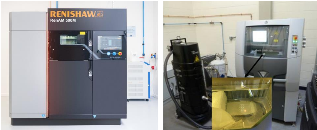
Figure 3-1. Renishaw RenAM 500M PBF-LB metal printer (left) for fabricating the Ti-6Al-4V alloys, 3D Systems ProX DMP 100 printer in NUI Galway (right) for 17-4PH SS, with inset image of view of build chamber during specimen fabrication.
