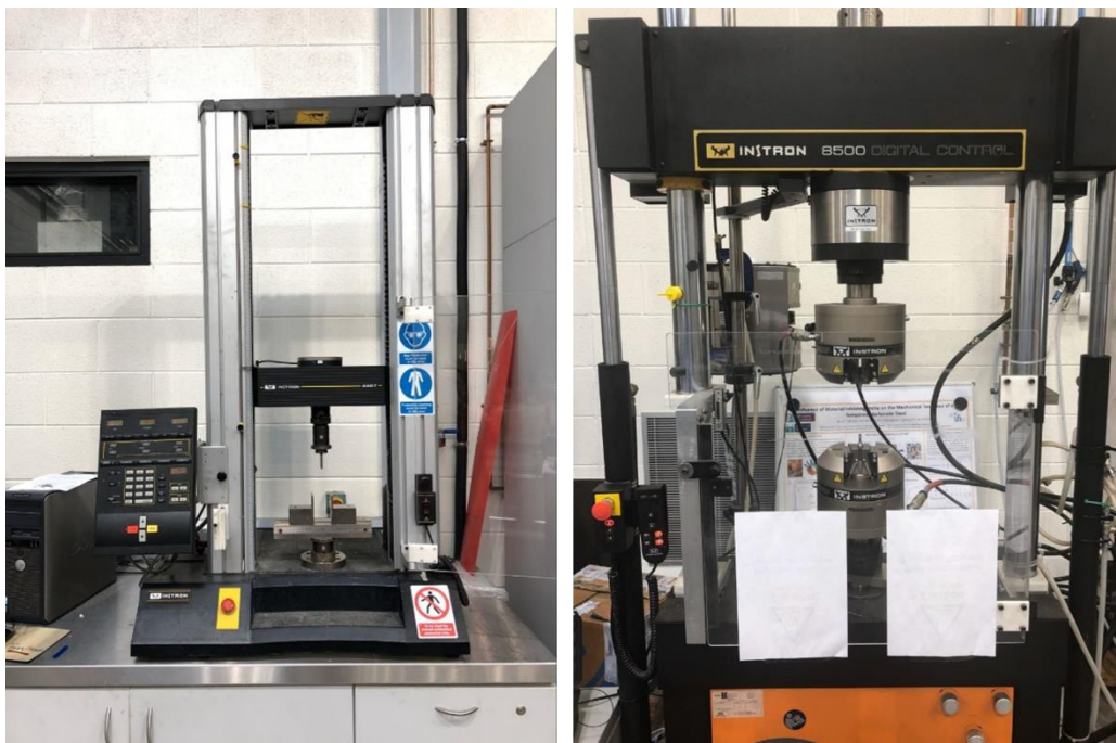
Figure 3-18. Instron 4467 (left) and 8500 hydraulic machines (right) for tensile and fatigue testing at NUI Galway.
