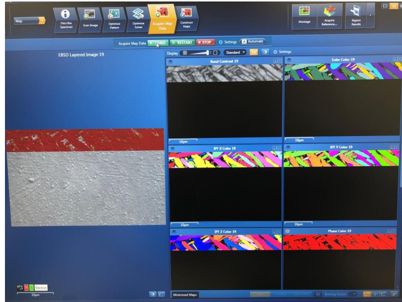
Figure 3-16. EBSD probe is indexing a PBF-LB Ti-6Al-4V scan, ~25% progress.
