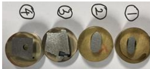
Figure 0-1. TiAl Etched samples, sample 1 (10 Seconds), 2 (15 Seconds), 3 (20 Seconds), 4 (25 Seconds).
