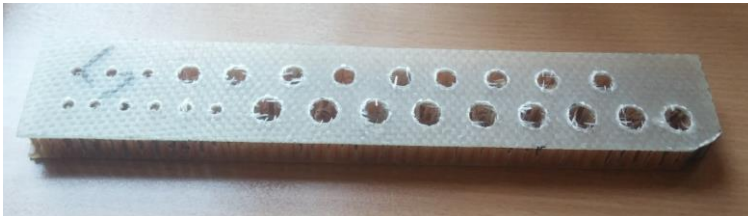
Fig. 2. Drilled holes with different diameter in sandwich composite sample.
