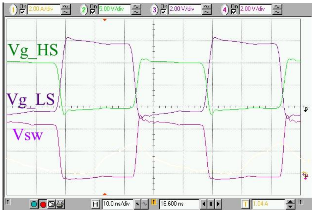
Fig. 5.14 Experimental waveforms with the 4thRes filter at V_{IN} = 4.5 V, V_{OUT} = 1.8 V, I_{OUT} = 2 A and F_{SW} = 20 MHz with 9-bit digital filter enabled, showing the high and low side FETs gate voltage ( V_{g\_HS} , V_{g\_LS} ), and switching node voltage ( V_{sw} ).
