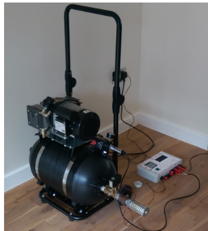
Figure 21 Setup of APU onsite
