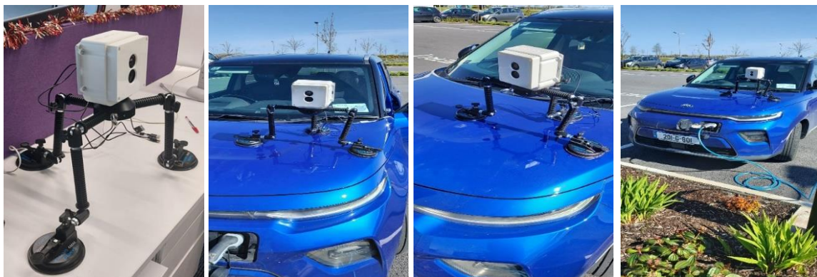
Figure 27: Thermal Data acquisition setup using M-2 method, housing case fixed on a tripod stand and tripod structure is placed on car bonnet with the help of suction cups.
