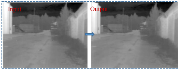
Fig. 6. Bad pixel replacement algorithm output on sample thermal frame, left side frame with some bad pixels and the right side is processed frame.
