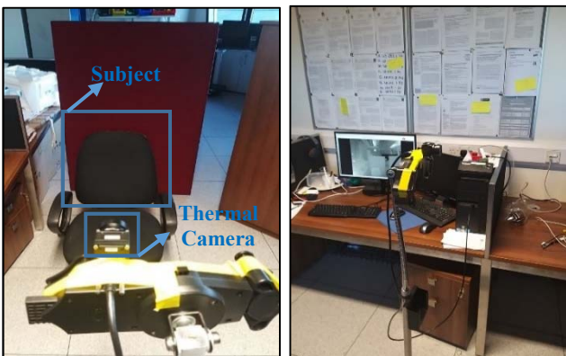
Fig. 8. Data acquisition setup in the indoor university lab environment, prototype thermal camera mounted on tripod stand placed at a fixed distance (nearly 60 centimeters) from the subject
