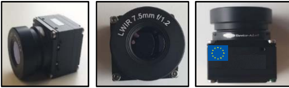
Fig. 7. Prototype thermal VGA camera model for acquiring local data
