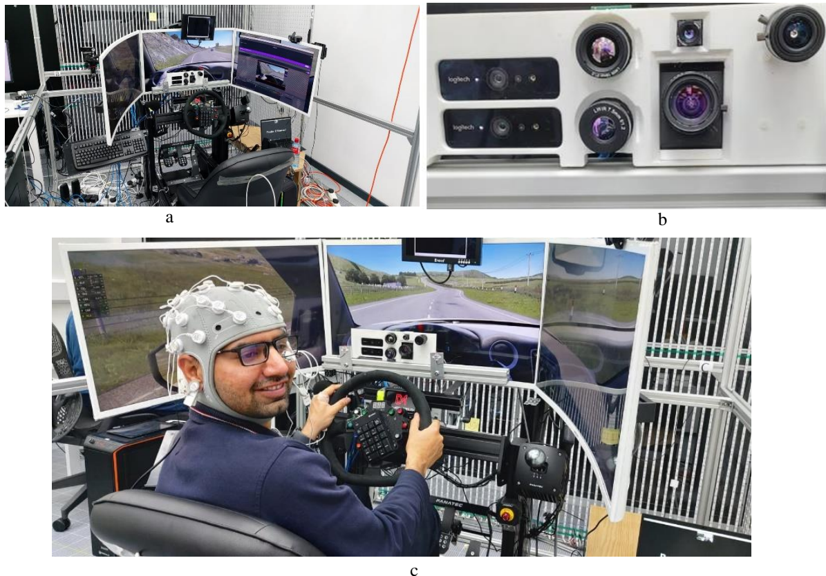
Figure 29: Data acquisition setup for drowsiness and cognitive load monitoring at XPERI Galway, a) Driving simulator setup with three wide angle monitor mounted for having real world driving experience, b) Different types of image sensors mounted at the center of middle display to record driver facial data, c) My self seated in the driver simulator wearing EEG, EOG, EDA, ECG, and SpO2 sensor kits.
