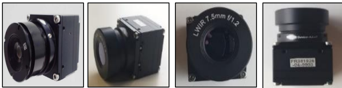
Figure 6: Uncooled LWIR 640X480 prototype thermal camera.
