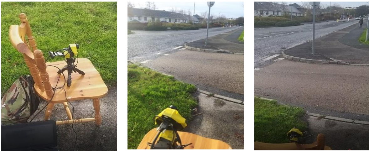
Figure 25: Thermal Data acquisition setup from roadside using M-1 approach such that by mounting the thermal camera at a fixed place.
