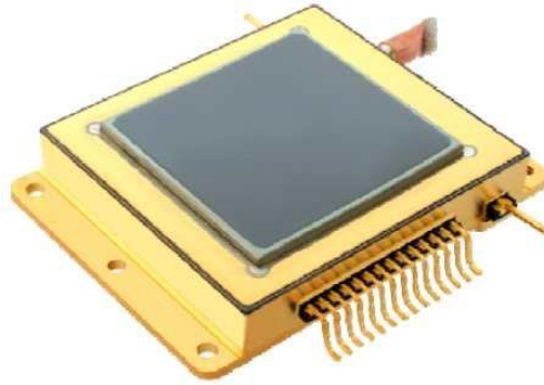
Figure 3: Microbolometer sensor array packaging [49].
