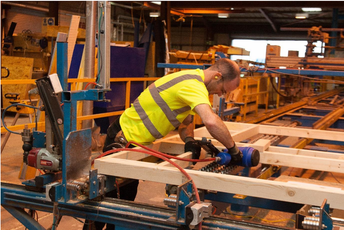
Figure 2-22: Panel assembly in Robertson Timber Engineering factory
