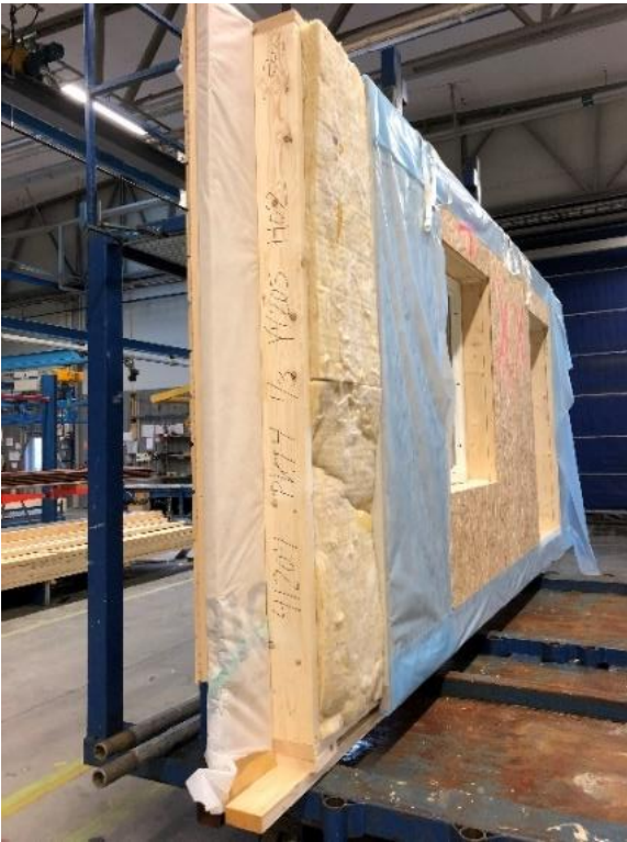
Figure 2-3: Derome Villa Anneberg wall panel loaded for transport at the manufacturing facility (image courtesy of Ylva Sandin).
