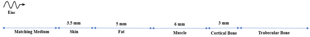
Figure 4.2: The 1-D planar layered model of the human heel, which is composed of five layers: skin, fat, muscle, cortical bone, and trabecular bone. E_{inc} is the probing wave.
