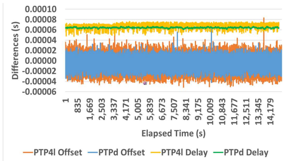
Figure 4-3. Offset and delay range of two PTP daemons running on the same machine.
