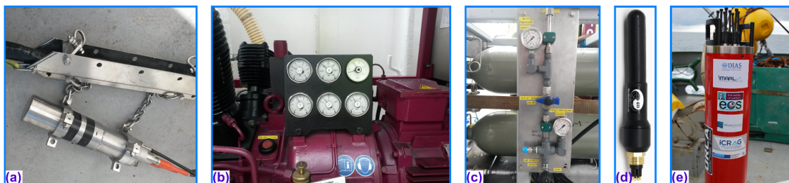
Fig. 3.4. Acoustic source and receiver equipment. (a) airgun and harness, (b) air compressor readout dials, (c) air collectors and dials, (d) GeoSpectrum M14-600 hydrophone (e) RS-ORCA acoustic recorder.
