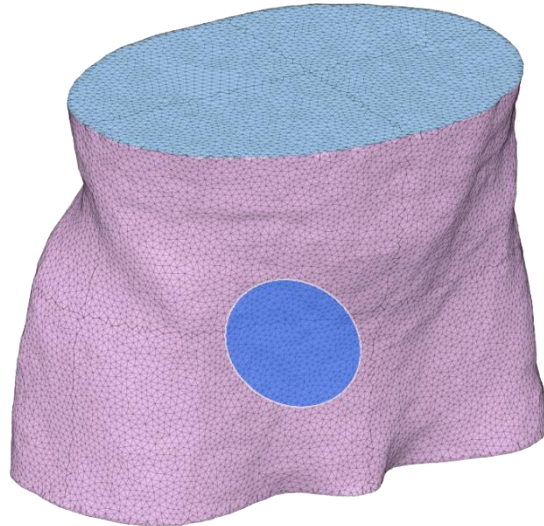
Figure 6.2: The realistic six-year-old model including the ellipsoid model in CAD format. The model is shown with a 60 ml ellipsoidal bladder (shown in blue). The model can be used for EIT data generation once the finite element mesh is created. However, additional tissues could be added to model such as bone.
