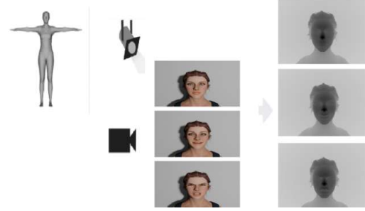
Fig. 8. Rendering configuration in Blender. The left row shows the body shape, light and camera setting; the middle row shows the facial RGB and the last row illustrates the corresponding facial depth image.
