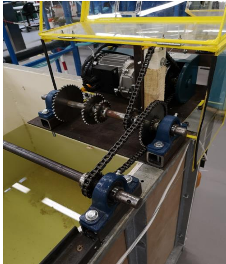
Figure 5-5: Towing tank motor showing the different gearing ratios for various tow speeds.
