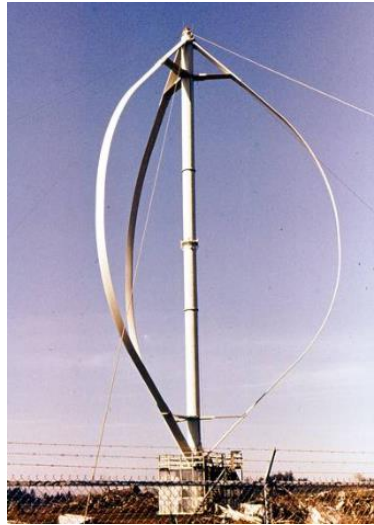
Figure 3-11: Three-bladed Darrieus wind turbine (Worstell, 1978).
