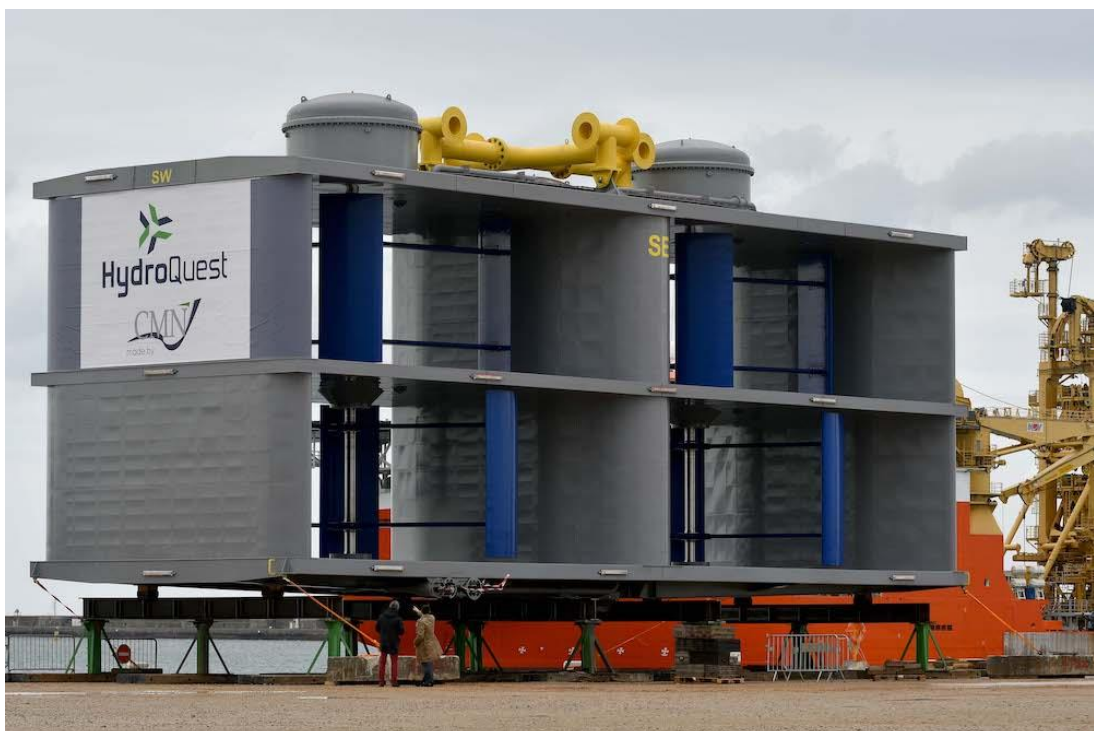
Figure 1-4: Hydroquest 1 MW OceanQuest prototype turbine device installed at Paimpol-Bréhat, France (HydroQuest, 2020).
