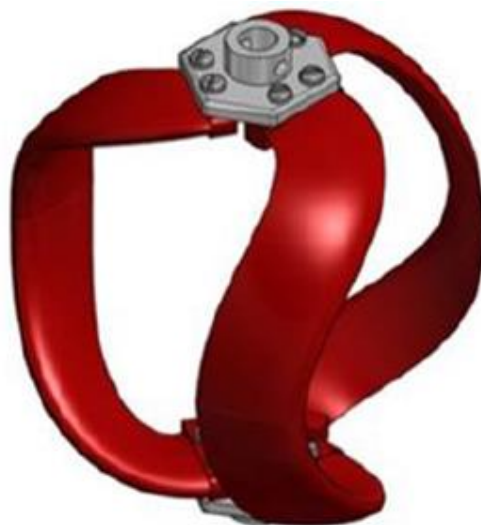
Figure 3-1: Brí Toinne Teoranta (BTT) design concept- Spherical/Ellipsoidal design.
