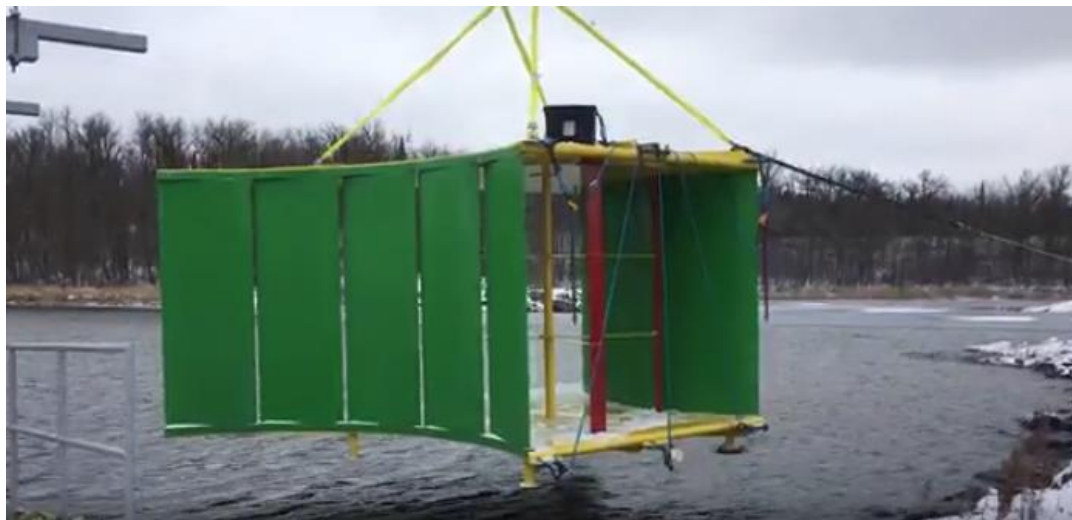
Figure 1-9: Davidson-Hill Venturi turbine (Tidal Energy Pty Ltd, 2013)
