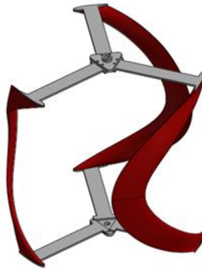
Figure 3-24: Brí Toinne Teoranta (BTT) design concept- cylindrical design.
