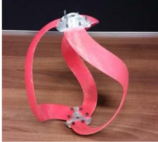
Figure 5-7: BTT scaled prototype tested in the tow tank
