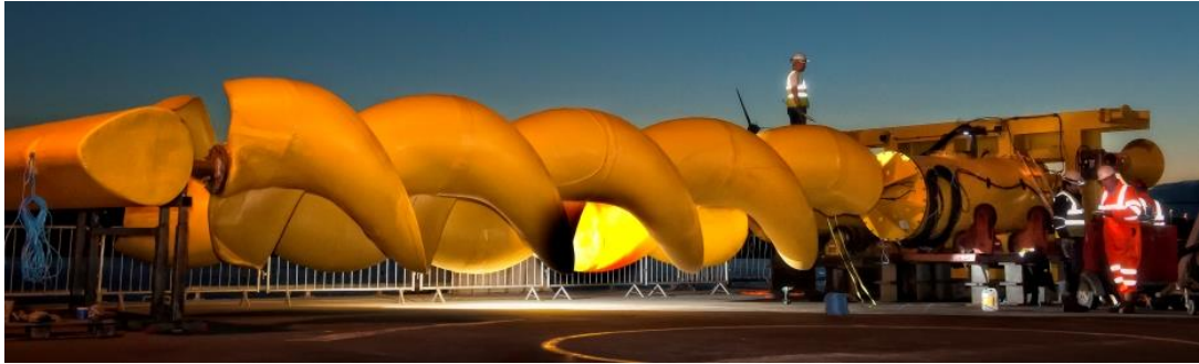
Figure 1-8: Flumill Archimedes screw turbine (European Marine Energy Centre 2020)
