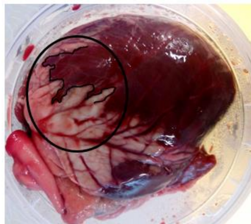
FIGURE 3. Lamb heart sample used to conduct dielectric measurements aimed at confirming the sensing radius calculated numerically. The area where measurements were performed is surrounded by a black circle and, within that area, the fat/muscle interface is marked.
