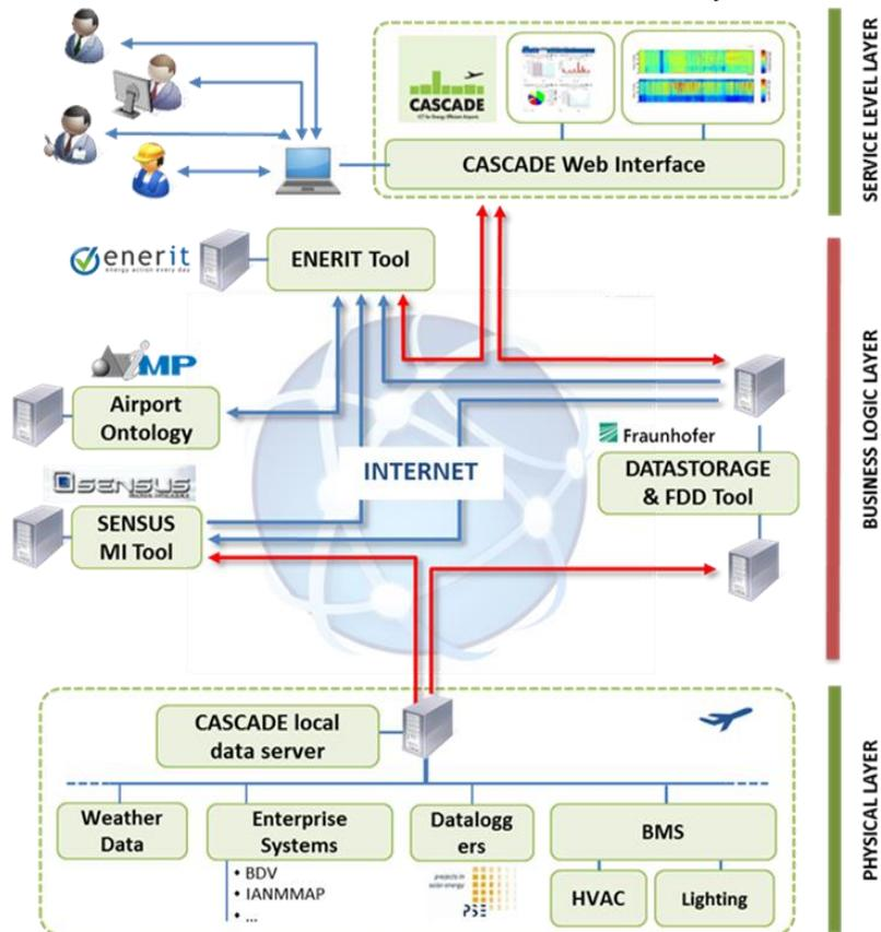
*Figure 2 The CASCADE Architecture*
