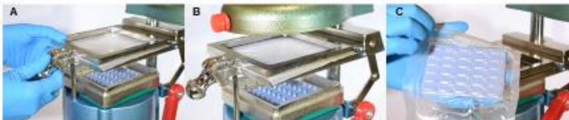
Figure 4.3 – Overview of thermoforming process. A) TPU is placed in the holder of the thermoformer. B) TPU film is heated by the heating element until it sags, the vacuum is turned on the TPU is pulled over the positive mold using a handle. C) Thermoformed TPU sheet on the positive mold.
