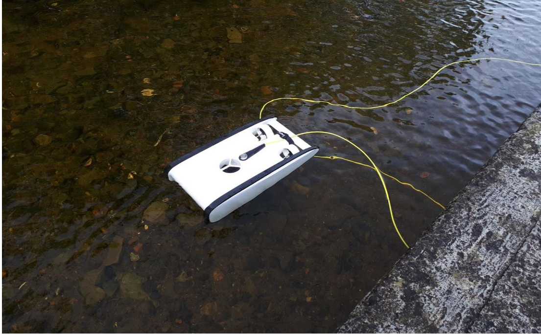
Fig. 5.2. Trident ROV undergoing freshwater trials using the 25 m tether.
