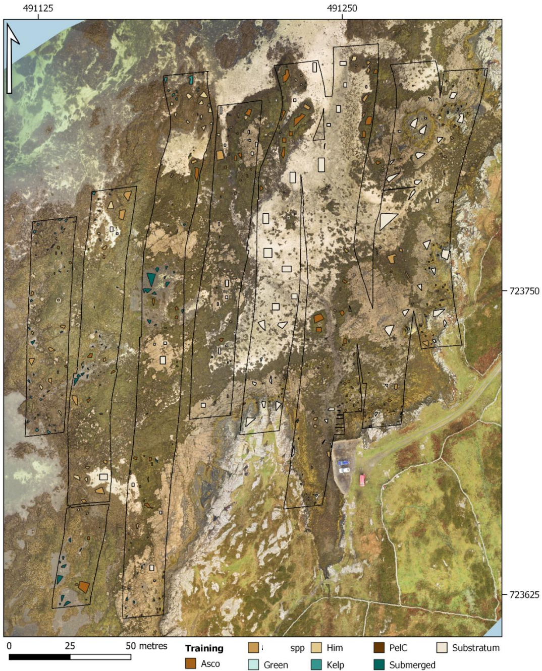
Fig. S3.3. Training polygons for all classes. The same class polygons were used for assessing the accuracy of both classifiers (MLC & SAM). The black lines mark the boundary of the hyperspectral data strips, and the background image is from the high resolution RGB UAV survey. Coordinates are in Irish Transverse Mercator (ITM). Class codes represent the following species. Ascophyllum nodosum (Asco), mixed fucoids ( Fucus spp), unidentified green species (Green), Himantalia elongata (Him), Laminaria digitata (Kelp), Pelvetia canaliculata (PelC), unidentified submerged macroalgae (Submerged), combined substratum (Substratum).
