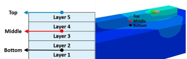
Fig. 1. The location of sample points from top, middle and bottom.
