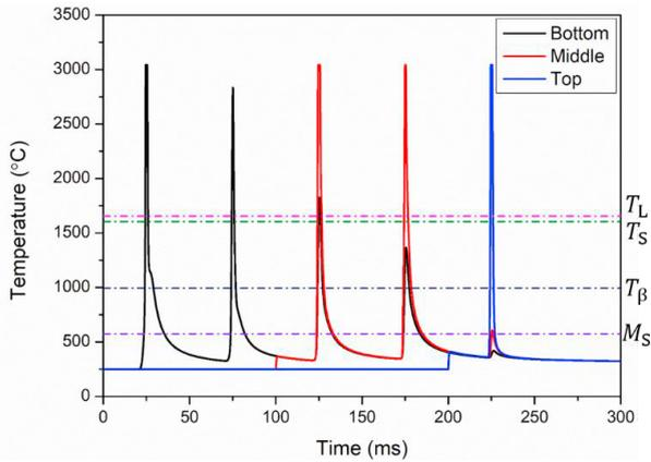
Fig. 2. Thermal history for the sample point during printing.
