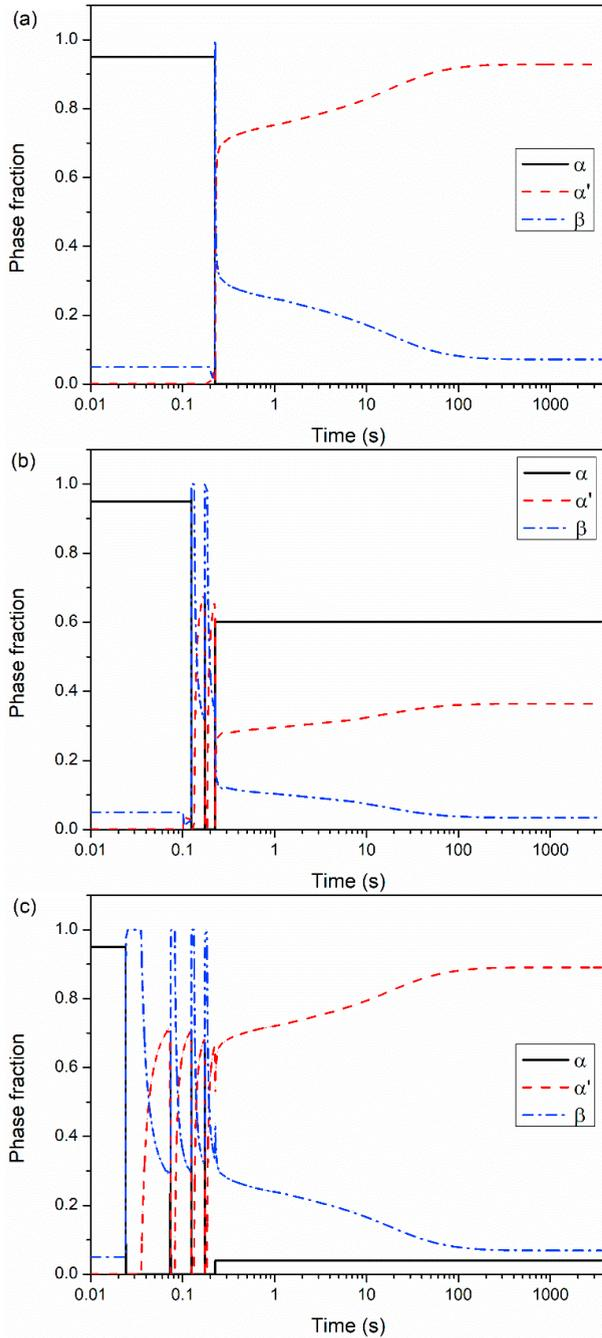
Fig. 4. Predicted phase fraction of  $\alpha$ ,  $\beta$  and  $\alpha'$  for the sample points (a) top; (b) middle; (c) bottom.
