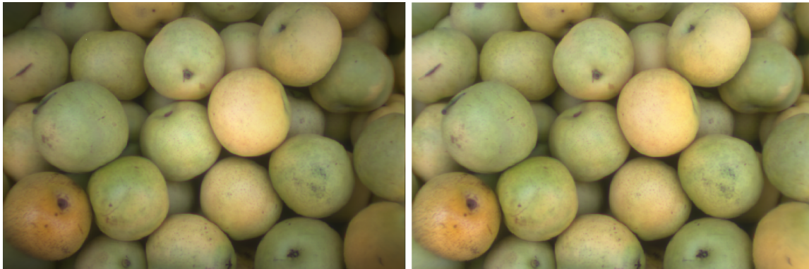
Figure 7.7: Vignetting for the proposed 1/3 inch sensor size format. On the left, the raw image, on the right, the corrected image both calculated using Zemax Image Simulation Toolbox.
