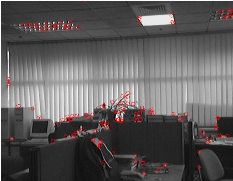
Figure 5.5: Example of SIFT features for an office image. Source: Engjw (CC by SA 3.0)
