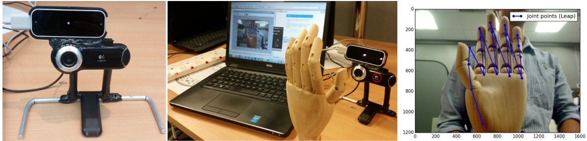
Fig. 4.8 Left : Webcam-Leap Motion setup used throughout the acquisition phase. Center : Example acquisition scenario using a dummy hand. Right : Coordinates outputted by the Leap Motion API, projected using the approach described in Section 4.3.4
