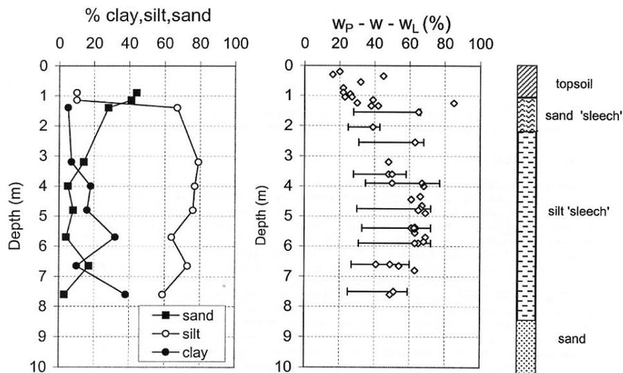
Figure 1. Stratigraphy at the Belfast test site
