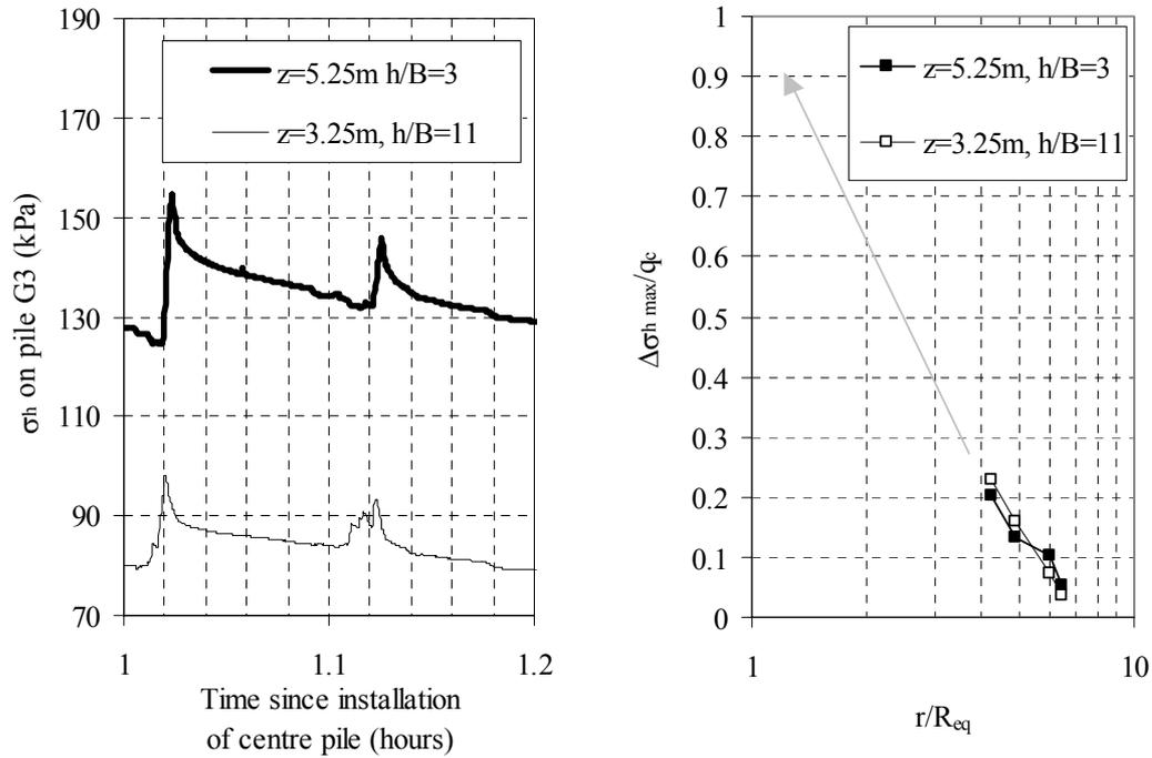
Figure 3. (a) Lateral stress changes on G3 during installation of G4 & G5, (b) Normalised maximum lateral stress changes associated with corner pile installations.
