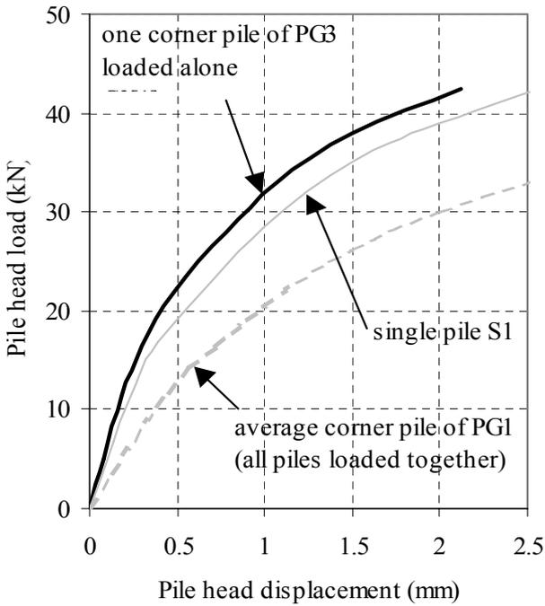
Figure 5. Response of corner pile in load tests
