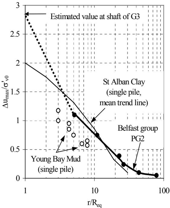
Figure 4. Radial variation of maximum excess pore pressures
