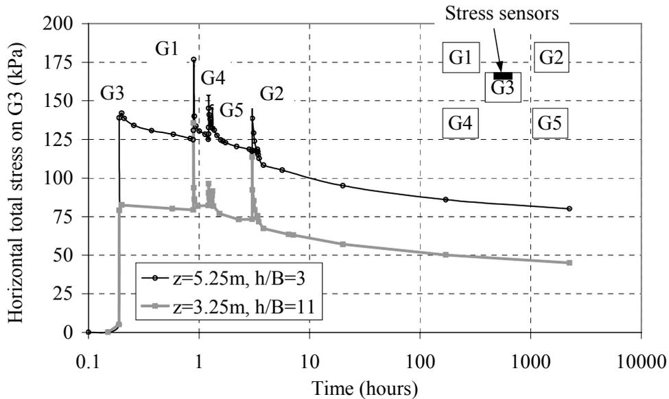
Figure 2. Lateral stress variations on centre of pile group during installation
