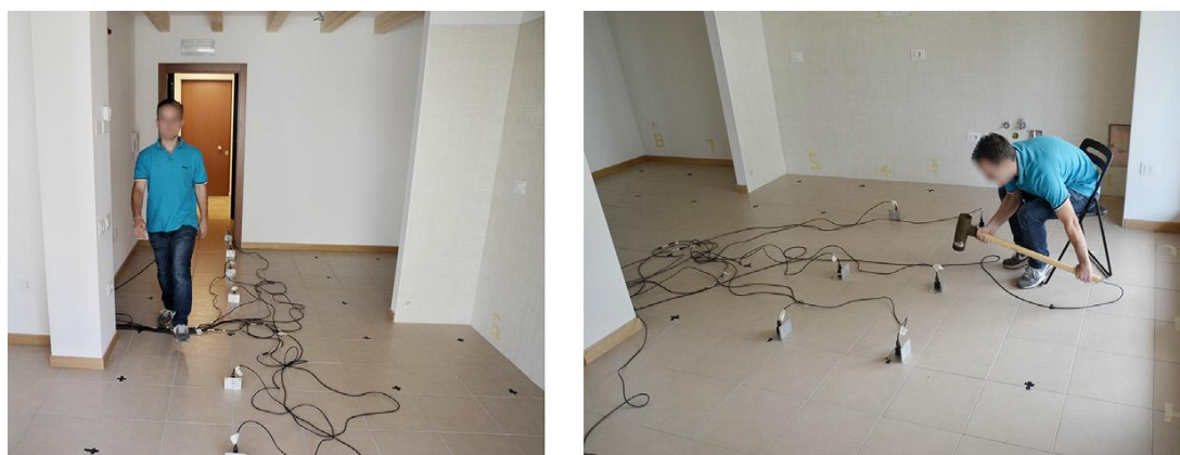
Figure 4.3 Walking and impulse hammer field tests on timber floors [132]
