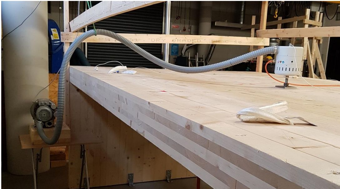
Figure 5.30 Electromagnetic shaker fixed to floor midspan, with cooling blower supported separately from the CLT test floor
