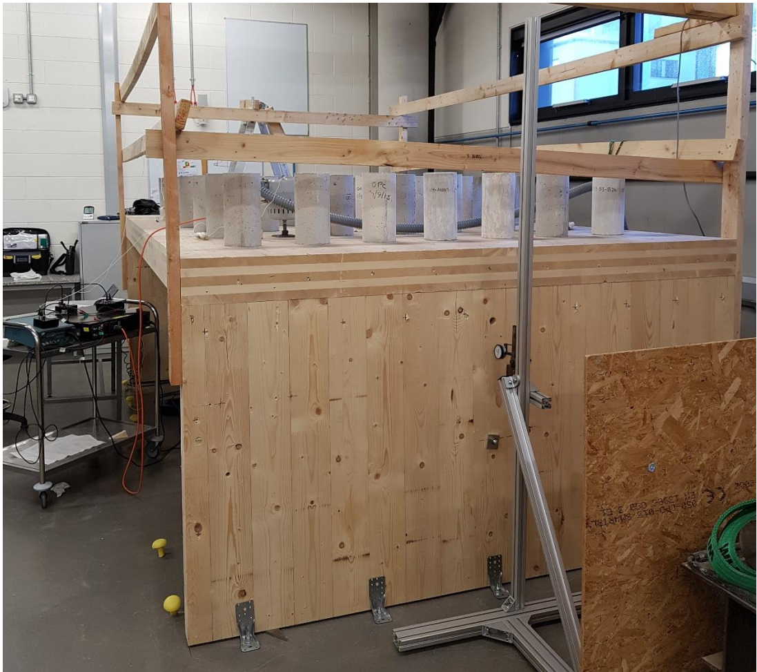
Figure 5.21 Long span platform construction dynamic testing with evenly distributed added mass, Assembly D
