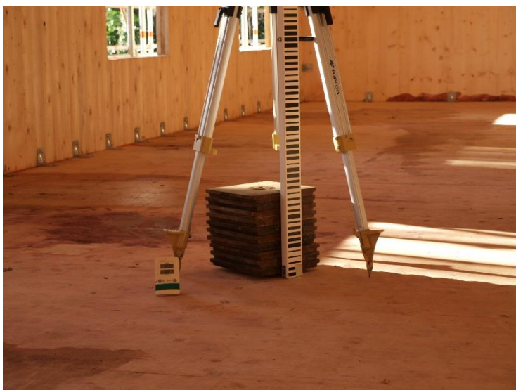
Figure 5.36 Static point load applied midspan
