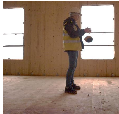
Figure 4.2 Impulse provided by a heavy rubber ball
