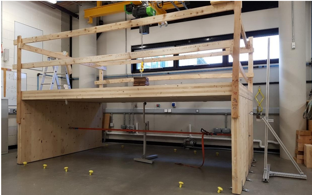
Figure 5.23 Static point load deflection measurement, one-way long span platform construction @ NUI Galway
