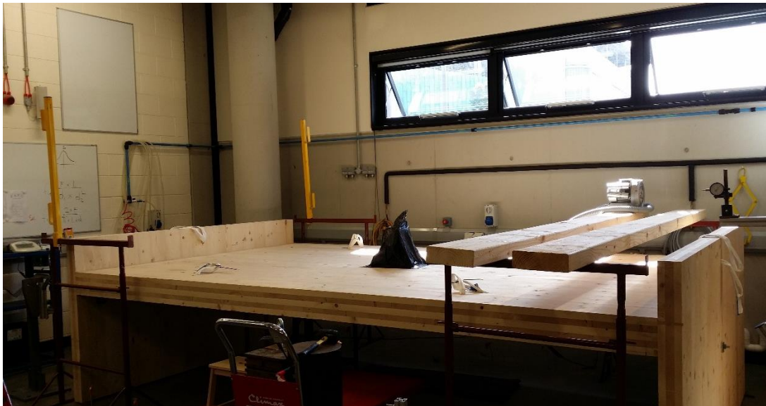
Figure 5.25 Independent scaffold erected for diagnostic impulse tests @ NUI Galway
