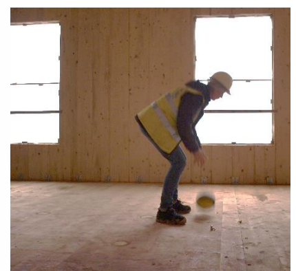
Figure 5.37 Impulse testing using a 2 kg ball
