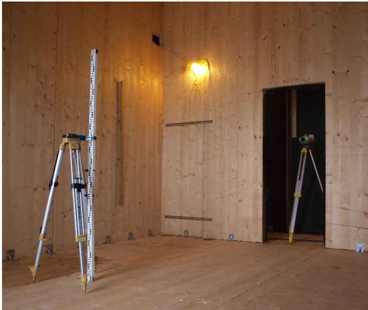
Figure 5.35 Static point load deflection testing
