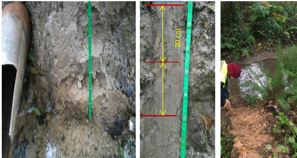
Figure 6.6. Bankside sampling with 30 cm intervals (left) after removing grass and plants (right).
