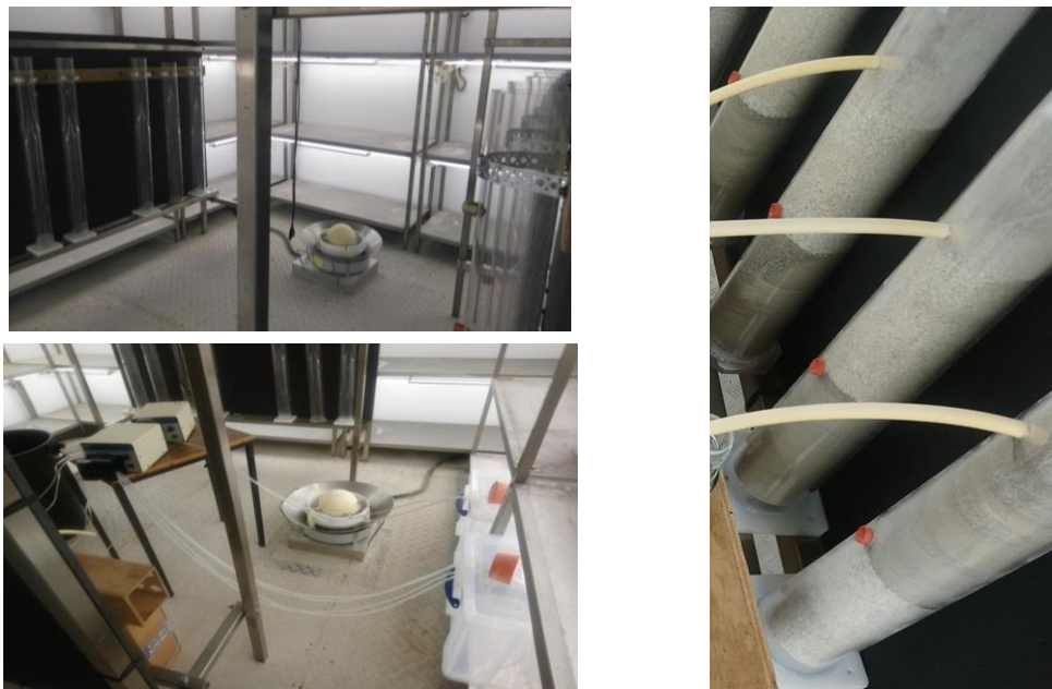
Figure 5.3. Large scale columns located in temperature-controlled room.
