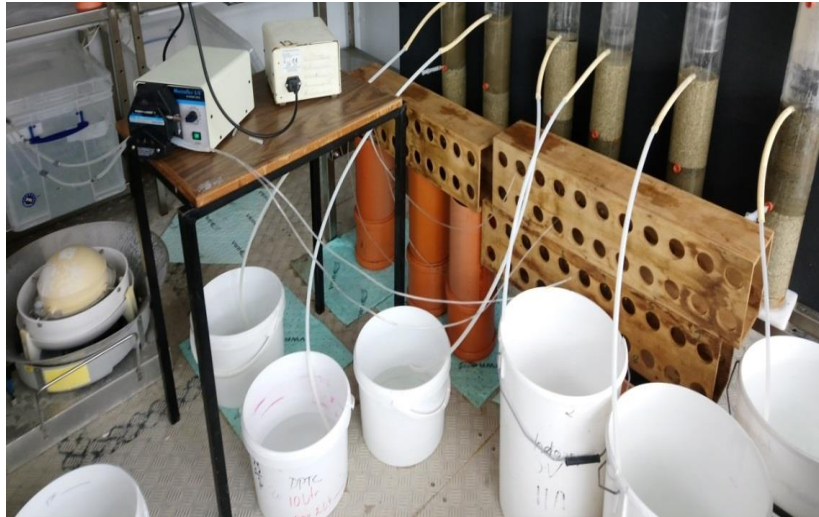
Figure 2.20. Space and required equipment to run large-scale column test. Johnstown Castle Research Centre, Co. Wexford.
