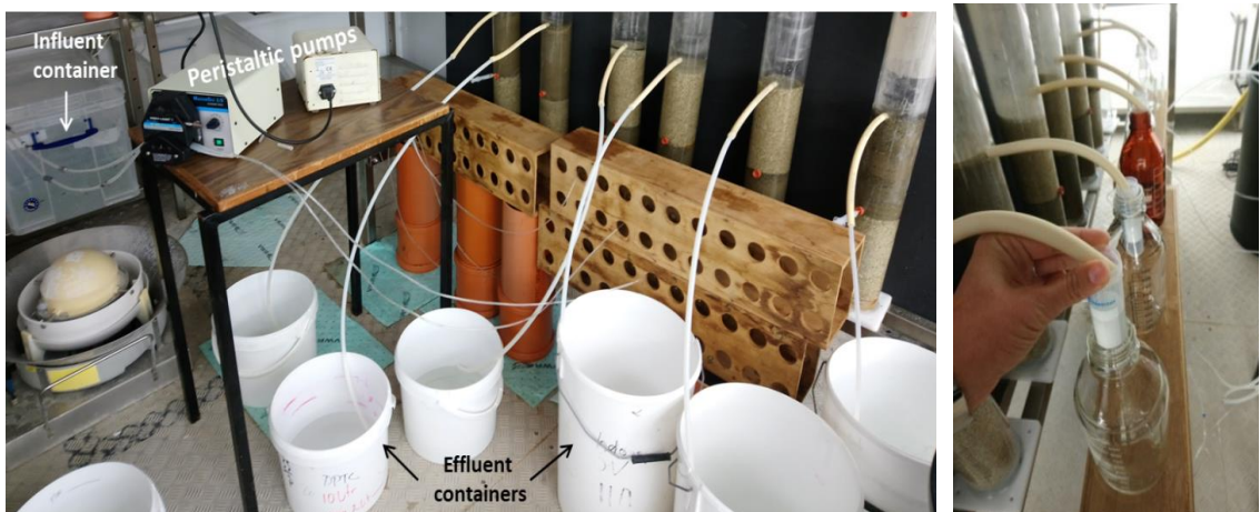
Figure 5.6. Large scale column operation (left) and sampling (right) from 6 columns packed with sand and zeolite in different configurations.
