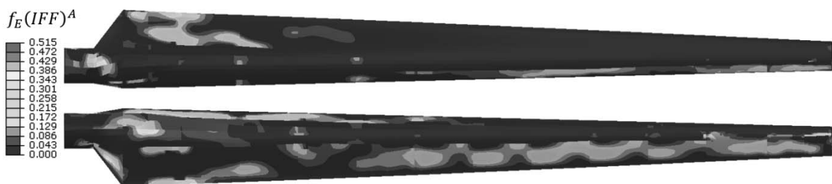
Figure 13. Contour plot of the stress exposure values for inter-fibre failure Mode A ( f_E(IFF)^A ) on the outer surface of the blade at the extreme wind load.
