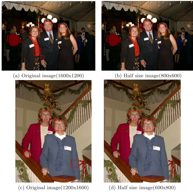
Figure 2.10: Eliminating false positives by resizing the images
