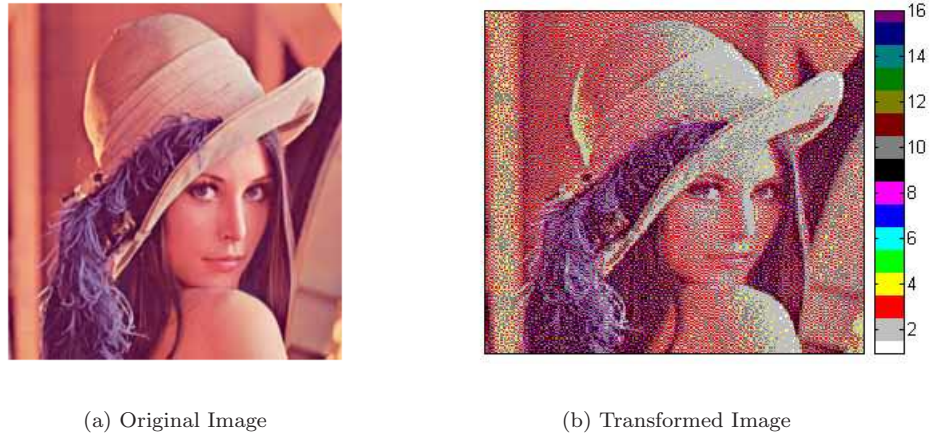
Figure 4.3: RGB to VGA colour transformation using dither
