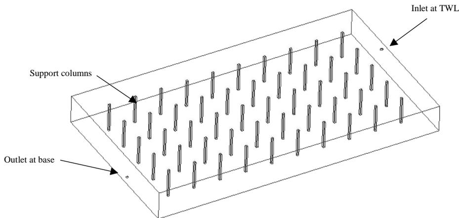
**Figure 1.** Schematic layout of the proposed service reservoir.
