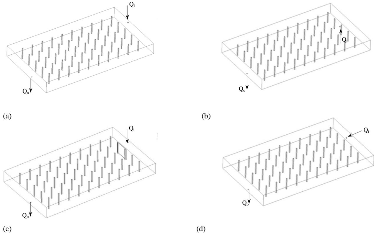
**Figure 2.** Schematic layout of each test scenario with  $Q_i$  showing the inlet location and direction and  $Q_o$  showing the outlet. (a) Scenario 1, (b) Scenario 2, (c) Scenario 3 and (d) Scenario 4.
