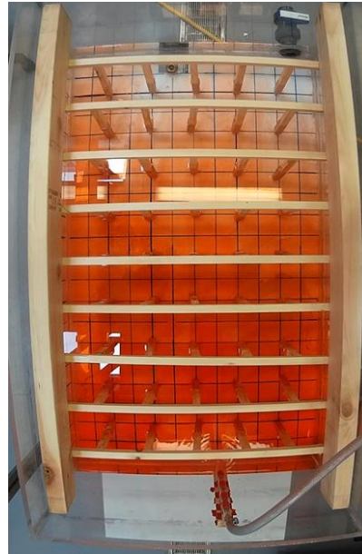
Figure 5. CFD volume rendering and food colouring test for time steps (a) t = 4 h (b) t = 10 h.
