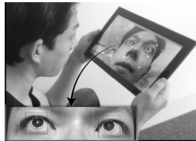
FIGURE 9. Eye tracking implemented in near real-time on a tablet. The tracking algorithm uses cascade classifiers and shape-based approaches to determine the eye region and centers. Elliptical model-fitting and 3D back-projections are then used to determine the eye optical axes and point-of-gaze [18].
