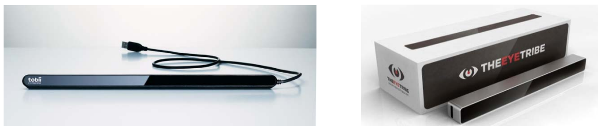
Figure K.1 The Tobii EyeX4C tracker (left) and the Eyetribe tracker (right)
