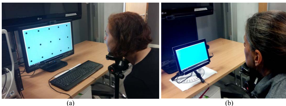
Figure 4.2: Gaze data collection setup showing eye tracker and UI on (a) desktop (b) tablet.
