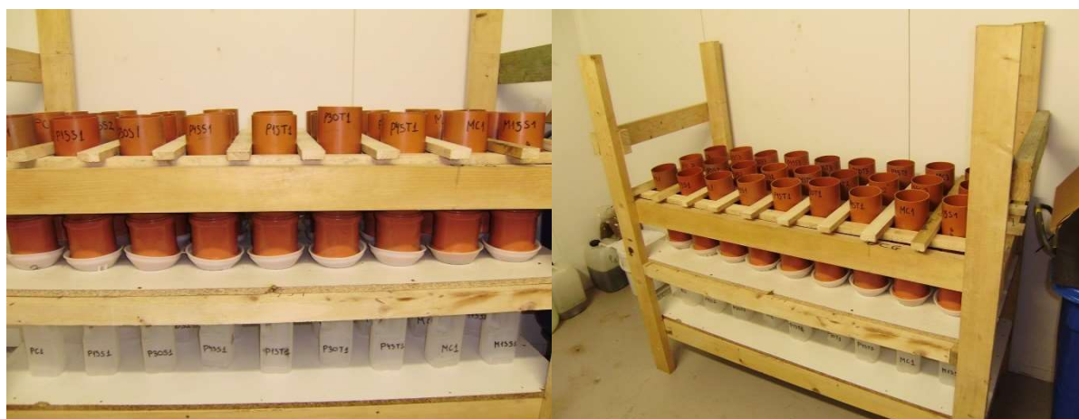
Figure 6.1. PVC columns containing packed soil
