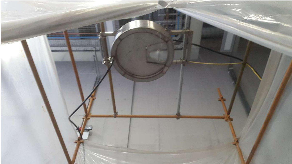
Figure 5.2. Rainfall simulator rotating disc.
