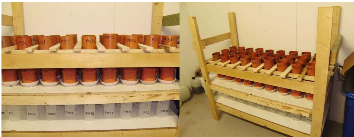
Figure 6.1. PVC columns containing packed soil
