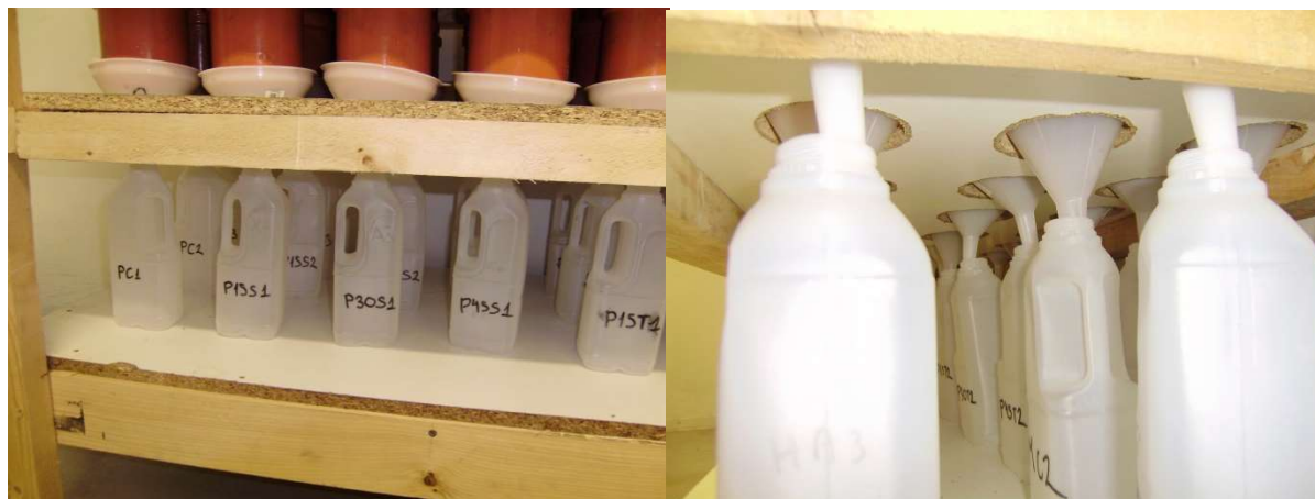
Figure 6.2. Containers and funnels used to weekly collect leached water.
