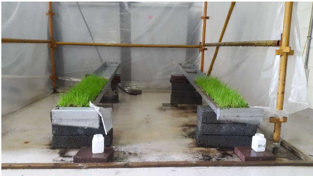
Figure 5.1. Flumes layout under the rainfall simulator.
