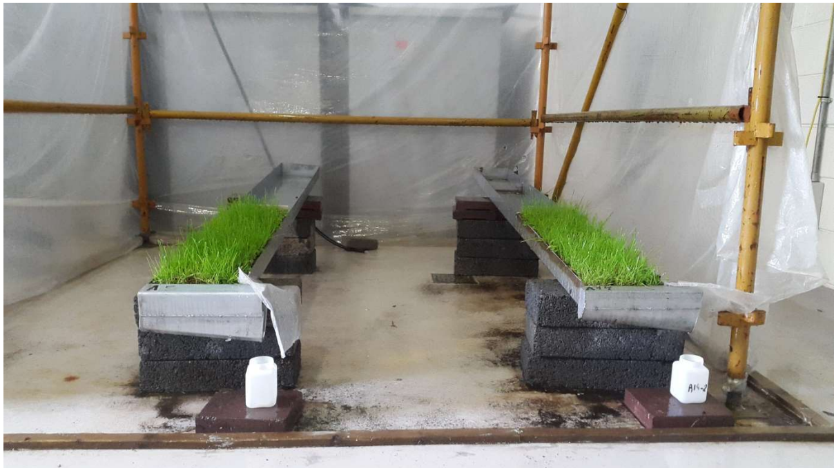
Figure 5.1. Flumes layout under the rainfall simulator.
