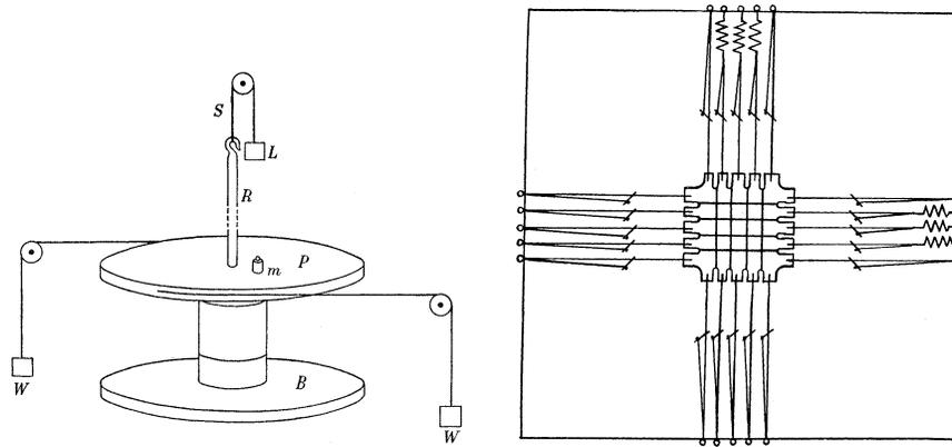
Figure 2: Rivlin was a very thorough and astute experimentalist. In one of his ten articles published from 1948 to 1955 in the *Philosophical Transactions*, he proposed protocols to measure the moment and normal force required to twist a rubber cylinder, and to measure stresses and strains in the bi-axial stretching of a rubber membrane [19].
