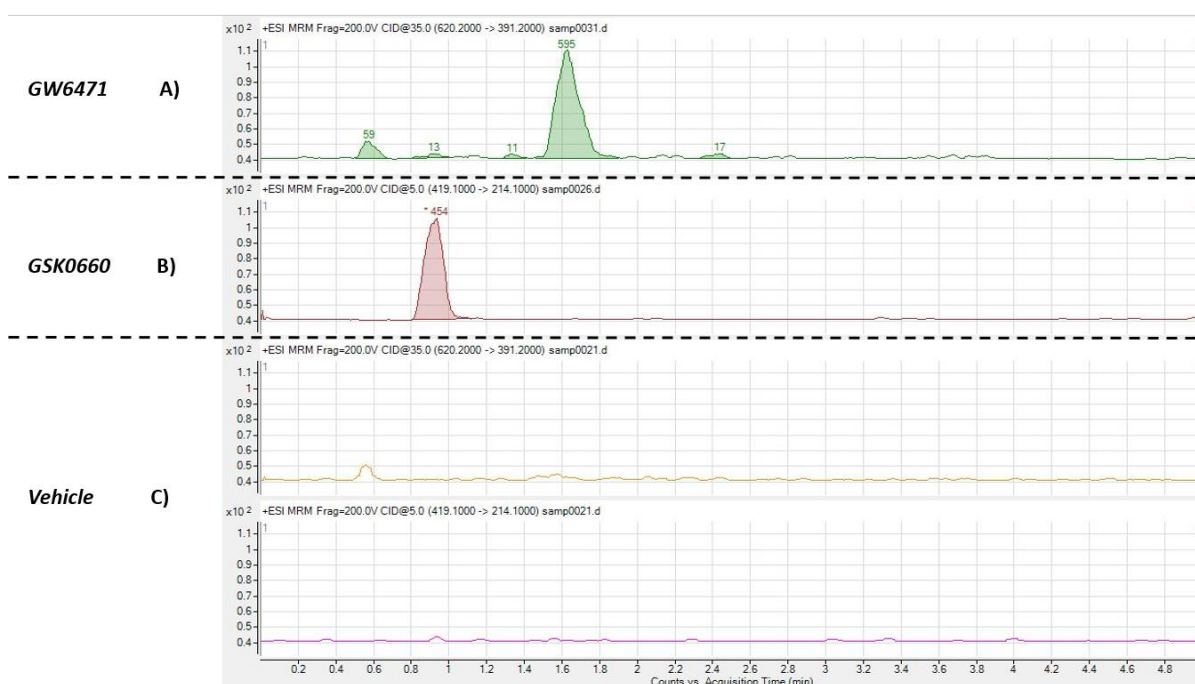
Figure 2.3: Detection of GW6471 (A) and GSK0660 (B) in DH punches. Analytes were detected using jet stream-positive ionisation with an Agilent triple quadrupole 6460 mass spectrometer interfaced with an Agilent 1100 HPLC system. The top chromatogram represents the detection of GW6471 at 620.2 to 391.2 m/z; the middle chromatogram represents the detection of GSK0660 at 419.0 to 214.0 m/z; the two bottom chromatograms represent the absence of the those transitions at the same retention times, indicating absence of the drugs (e.g. vehicle-treated subjects).
