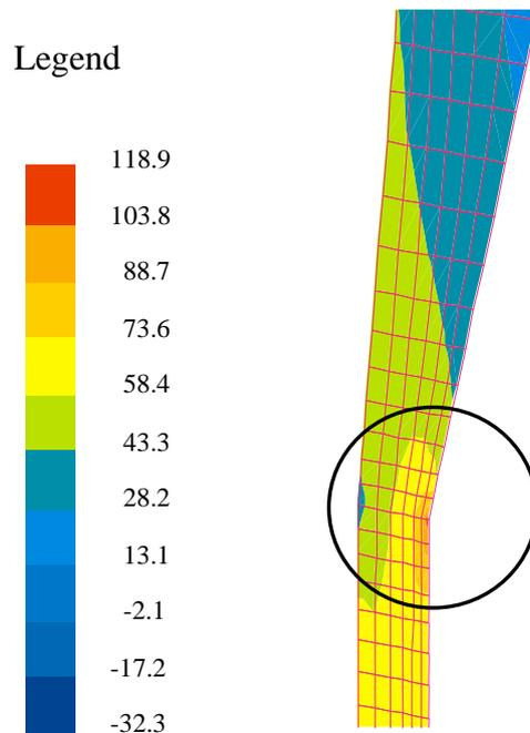
Fig. 6. Axial stress (MPa) contour plot in area of transition from pipe to female section
