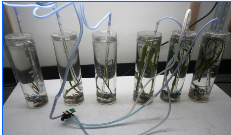
Fig. 6.1 Image of the experimental design of one temperature treatment with shoots from the Irish population of Zostera marina . Each cylinder ( n = 3 ) contained 3 shoots and had a volume of 3 L and a height of 35 cm.
