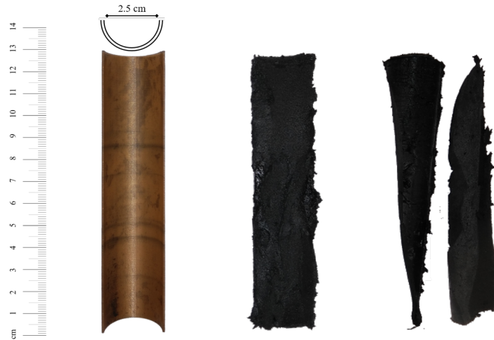
Figure 3.5: Glandular tissue construction. The half-cylindrical mould used to fabricate the glandular tissue is displayed on the left. An example of an uncut glandular piece is then shown in the middle, and the two resultant cones are shown on the right.
