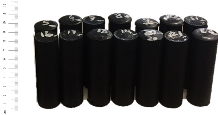
Figure 3.8: Example of some of the tumour plugs to be used in combination with the breast phantoms. All plugs have an indication of “rotation 0” on the top.
