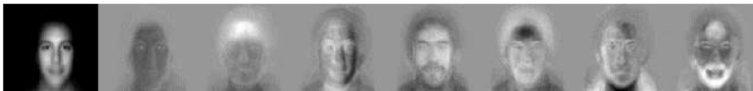
Figure 2.6. Eigenfaces, as presented in [19]: the average face on the left, followed by seven top eigenfaces.
