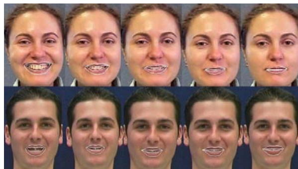
Figure 7.8. Example of mouth tracking sequences: the first row contains results from one of our video sequences, while in the second row there are exemplified frames from the VidTIMIT database.
