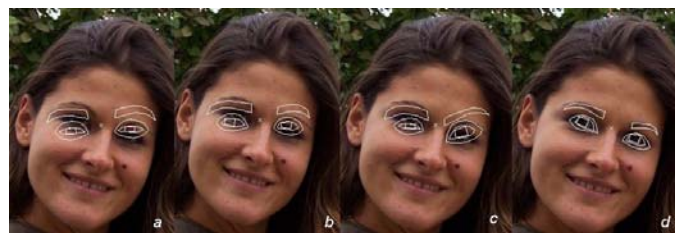
Figure 7.2. From left to right: a. the initialisation of the eye-shape inferred from face detection; b. the eye-shape from global AAM fitting; c. the eye-shape from AAM sub-model fitting; d. the fitted shapes of the component sub-models refitted by the global AAM – note how the two eyes are constrained into a two-eye limit.
