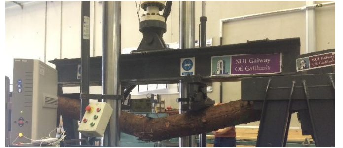
Figure 1: Four point bending test setup
