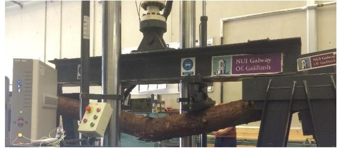
Figure 1: Four point bending test setup
