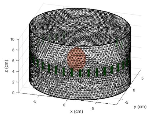
Fig. 1. Simulation FEM for data generation. Within the FEM, the bladder (orange) is represented as an ellipsoid that ascends vertically, mimicking the urinary bladder in the pelvic cavity. The electrode positions are shown as green rectangles.
