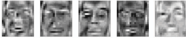
Figure 2: Examples of lower order eigenface Vectors
