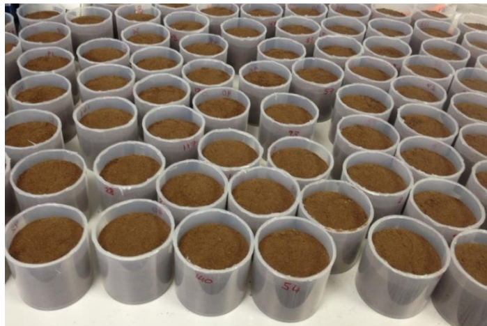
Figure 4.1. Microcosms constructed from plastic containers, filled with sieved soil at a bulk density of 0.77 g / cm 3
