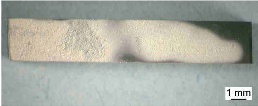
Figure 15: Macroscopic view of MoSi 2 /HfO 2 (series I2b) after 500 h at 500 °C in air: thin yellow layer consisting of MoO 3 crystals and SiO 2 clusters
