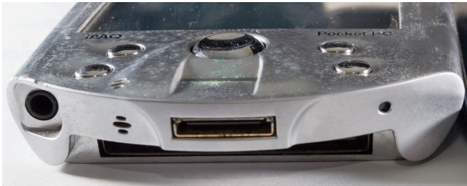
Fig. 2. A close-up of the swipe fingerprint sensor (below the main central button) on an older IPaq handheld computer.
