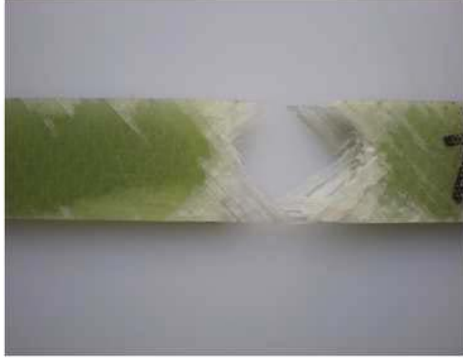
0.85% Initial strain, R = 0.1 # of cycles to failure 8,130,871 (b)
