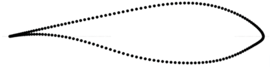
Figure 5 Cross section view of RISO-A1-24 airfoil
