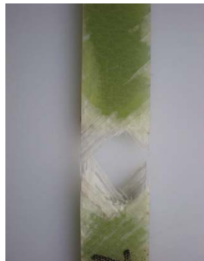
0.85% Initial strain, R = 0.1 # of cycles to failure 8,130,871 (b)
