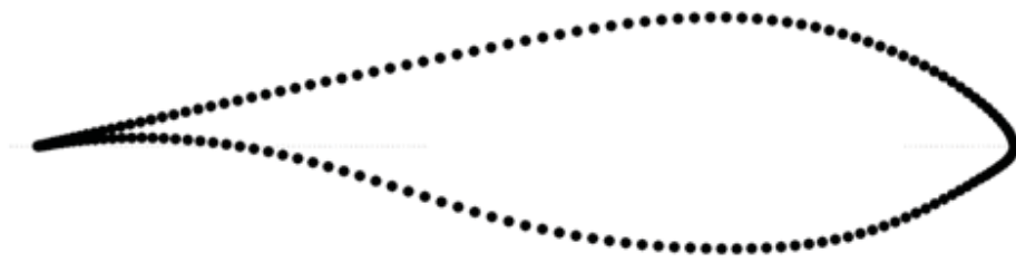
Figure 5 Cross section view of RISO-A1-24 airfoil
