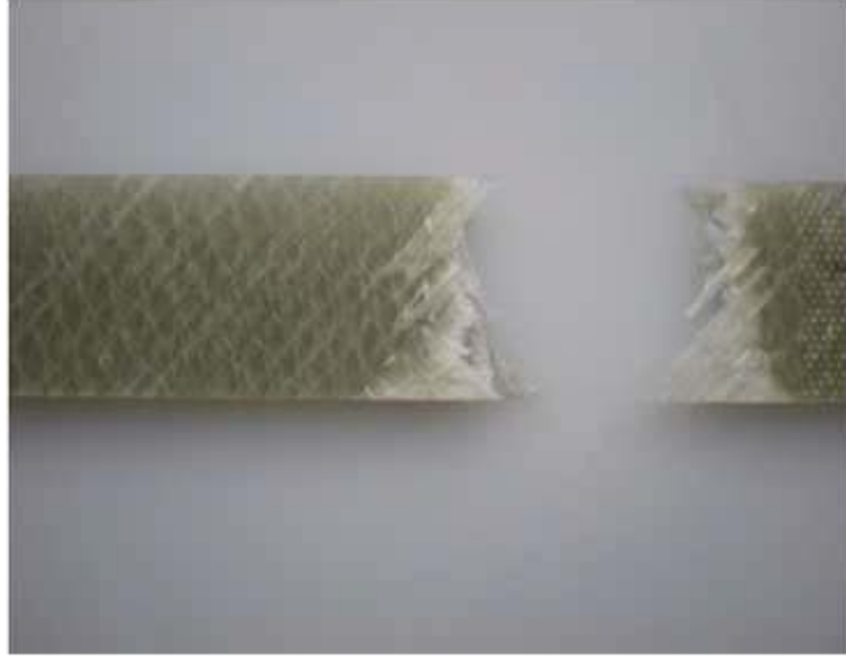
0.81% Initial strain, R = 0.1 # of cycles to failure 52,041 (a)
