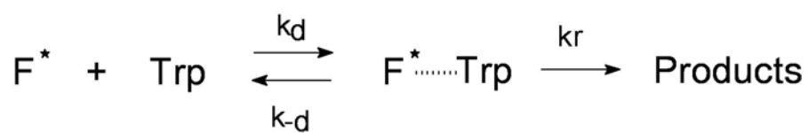
SCHEME 2 – Bimolecular fluorescence quenching mechanisms.
