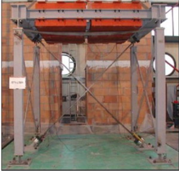
Fig. 2. View of test frame on shake table prior to testing.
