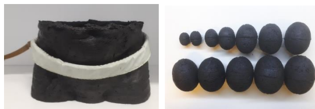
Figure 3: (left) Conductively and anatomically-accurate male child-sized pelvic phantom for EIT as presented in (Dunne et al 2018b). The internal conductivities are modelled as a weighted average of all pelvic organs ( 0.2 \text{ S m}^{-1} ). This region is realized using ultrasound gel with additional sodium chloride. (right) The employed bladder phantoms, ranging from 40-380 ml.
